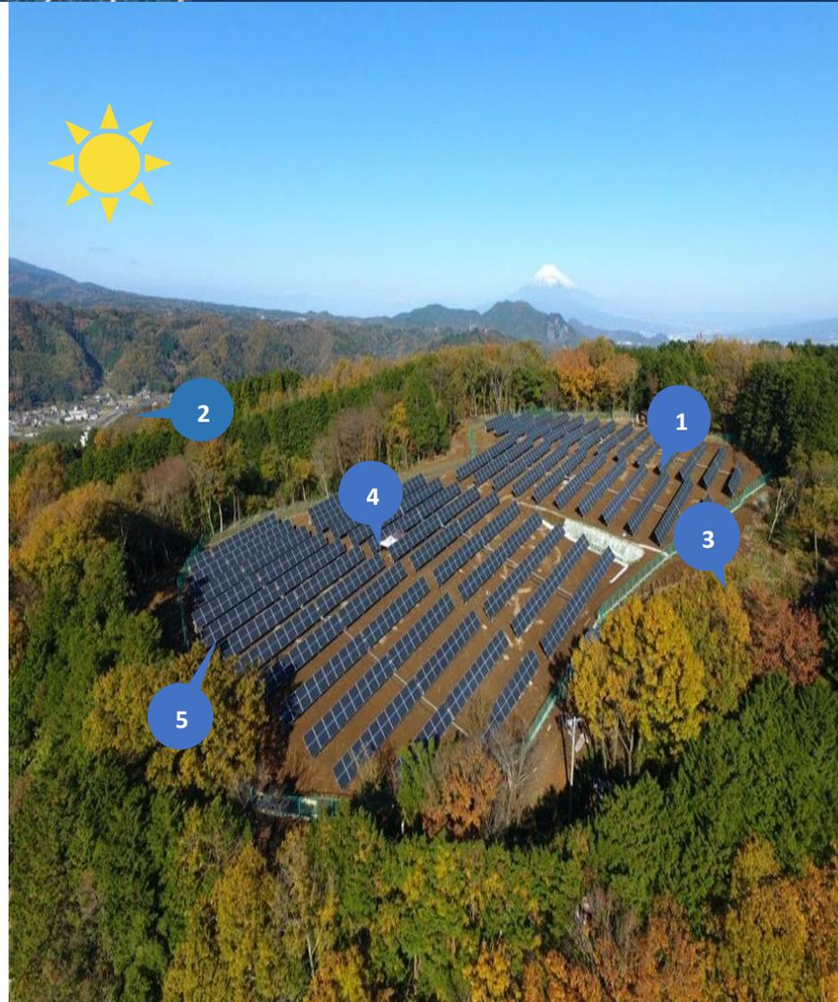
**4 Topography:** Solar best fits land that slopes less than 10% and is south-facing towards the sun. We will walk the land to get a sense of the topography and where the installation is best placed. Flatter land also allows for a wider range of solar technologies to be developed on-site, including single-axis tracking systems.
